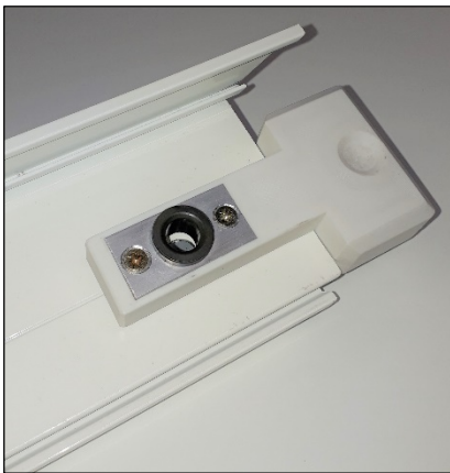
Positioning of the drilling template on the cut profile at 45°
